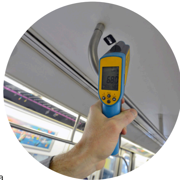
Technician collects temperature data on subway car while testing HVAC systems
